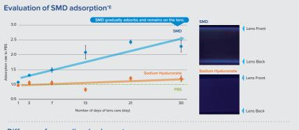
\*E Test method: Silicone hydrogel lenses are immersed in fluorescent-labeled sodium hyaluronate or hyaluronate derivatives for 8 hours, and in ISO-PBS overnight. The volume of each adsorbed ingredient is measured after repeating this procedure 30 times, and the adsorption is observed under a confocal laser scanning microscope.
